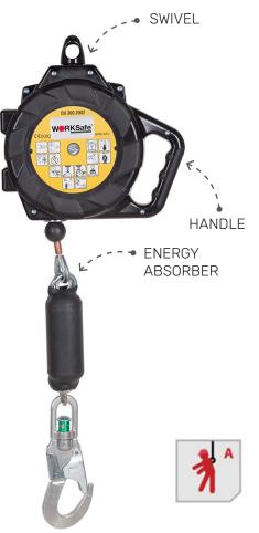
CR 250H + V self-locking device for vertical and horizontal operation in a plastic casing with a pull-down steel rope and a swivel mounted in the casing. The device has an additional shock-absorbing system located near the snap-hook. It is intended for work requiring considerable displacement in relation to the point of attachment. A safety shock absorber is not required. Also, the AZ 800 cable is not needed when working horizontally. Available in 6m, 8m and 11m.
